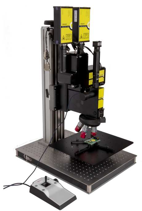
Fig. 1. Riscure's double laser injection system
